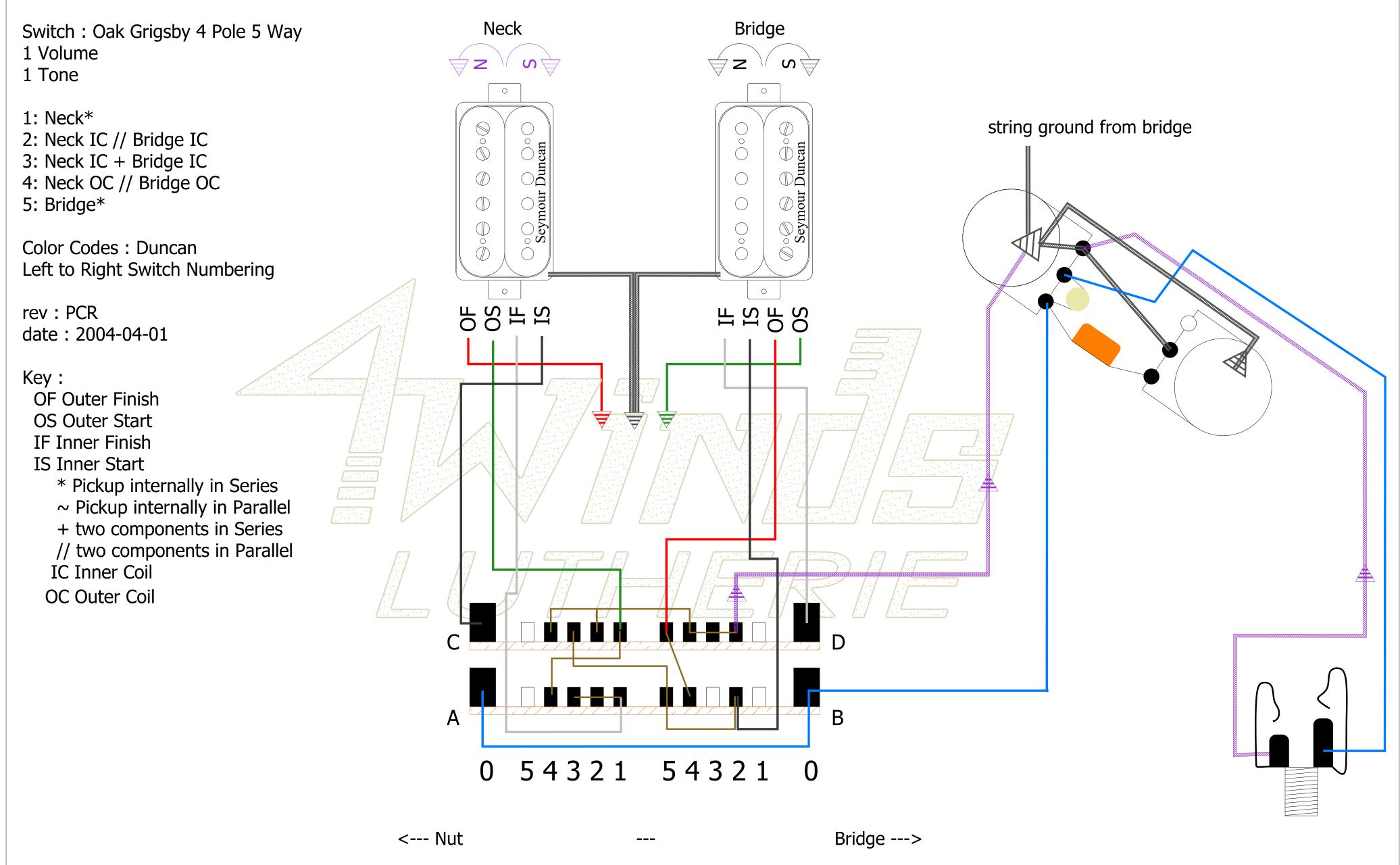
\*Note 0: This diagram ports stock mid-90's to mid-00's 5 Way Rotary sounds to a blade form factor with 4 conductor pickups \*Note 1: Neck pickup magnet flipped 180° to achieve inner slug coil South polarity
