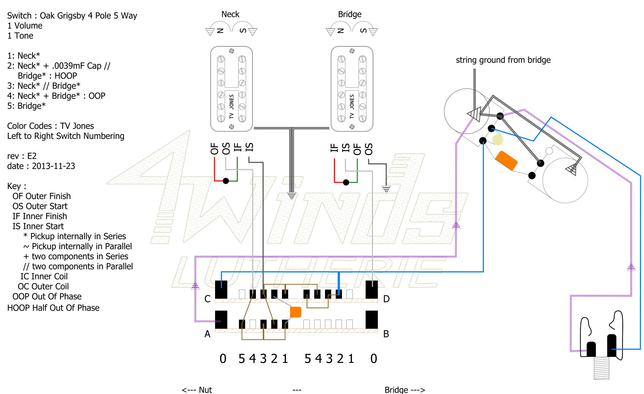
\*Note 1: Although shown with 4 conductor wire, this circuit does not utilize the series join leads for switching. Therefore this scheme can be adapted to any 2 pickup layout including single coils. Pickups with baseplate or cover internally connected to the coil ground lead, such as Telecaster or P-90, must be modified to add a 3rd lead to ground the metal components separately.
