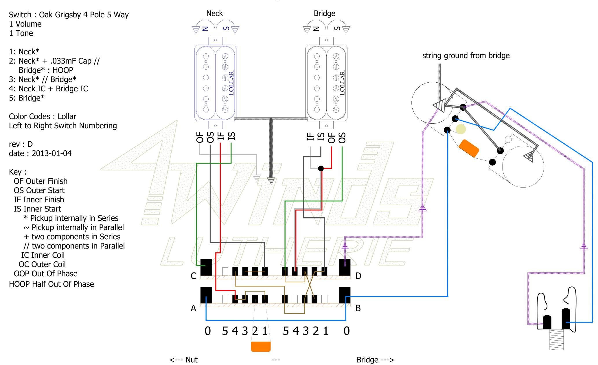
\*Note 1: Neck pickup *rotated 180°* to achieve inner Screw coil South polarity
