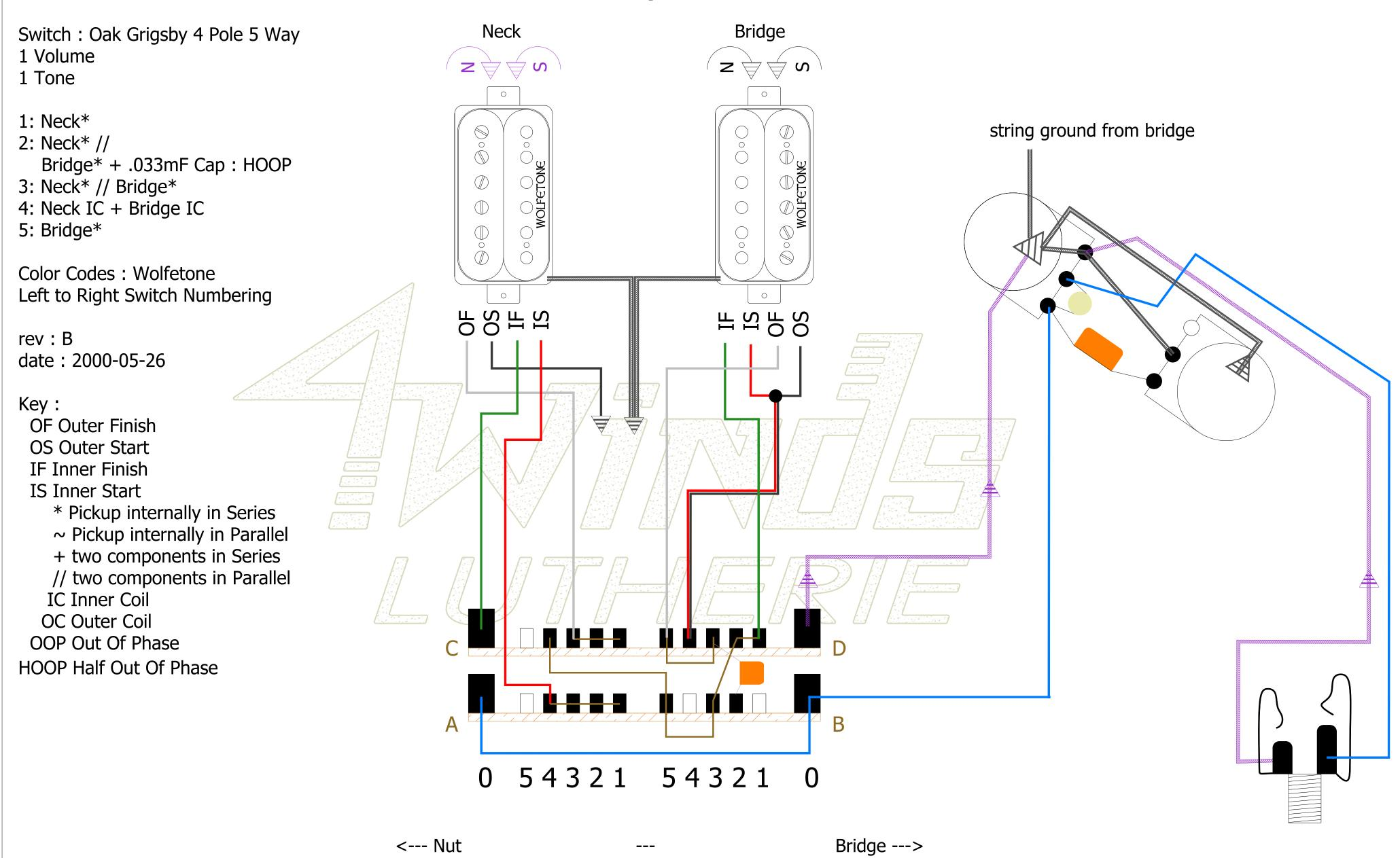
\*Note 1: Neck pickup magnet flipped 180° to achieve inner slug coil South polarity
